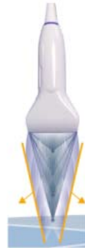
Radiation force created by SonicTouch™. The shear wave is amplified along a Mach cone (yellow). The distance traveled is increased, thus minimizing acoustic energy used.
